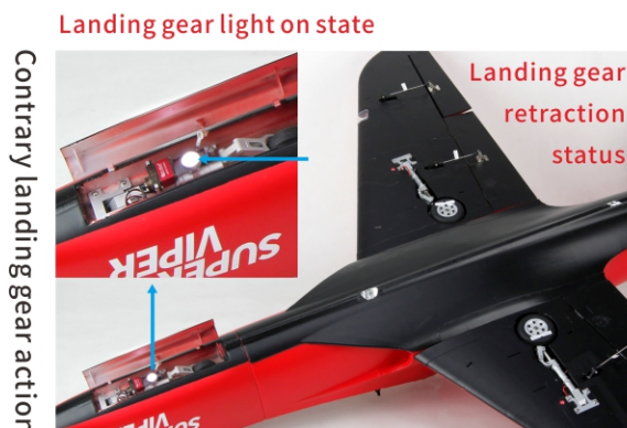
Possible landing gear reverse action
